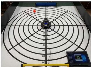
Center the robot in the measurement field
